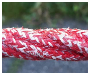
Longer-term operation: Diameter in the knot area is reduced, first mono- and multifilaments wear out
