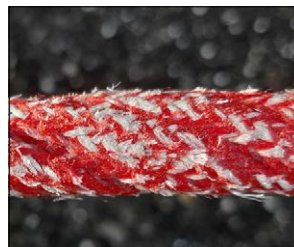
Schedule rope change: Diameter in the knot area is strongly reduced, knot structure becomes indistinct, all visible fibers with wear
