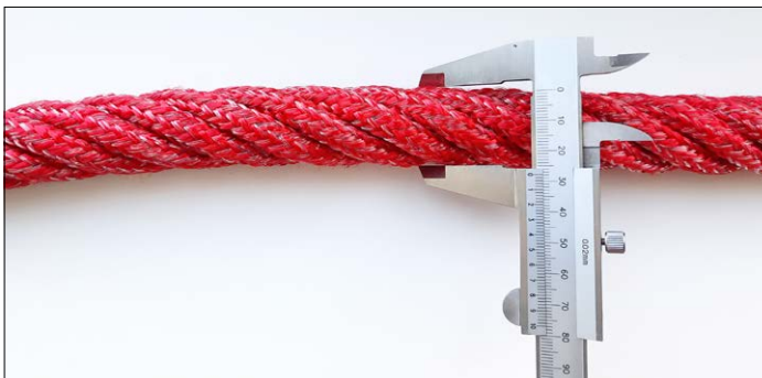
Figure 9: Caliper gauge lying flat for correct determination of the rope diameter
