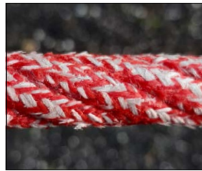
Schedule rope change: all visible fibers with wear
