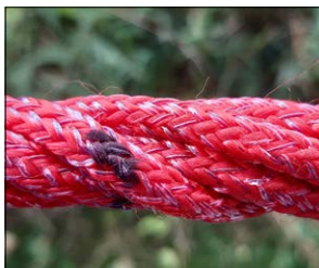
Start of operation: Knot structure as well as Mono- and multifilaments intact
